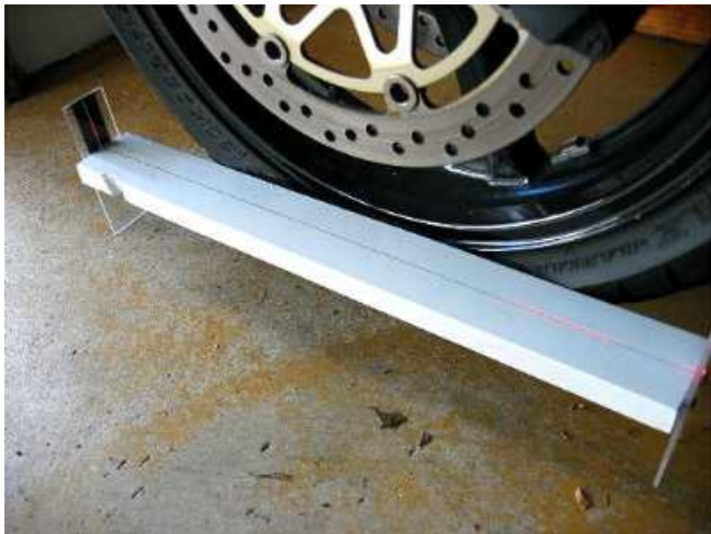
Illustration 7 – laser beam running parallel to centre line
