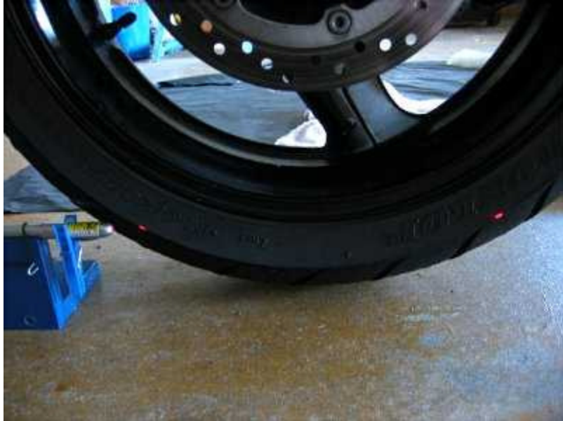
Illustration 6 – laser beam touching tyre at 2 points
